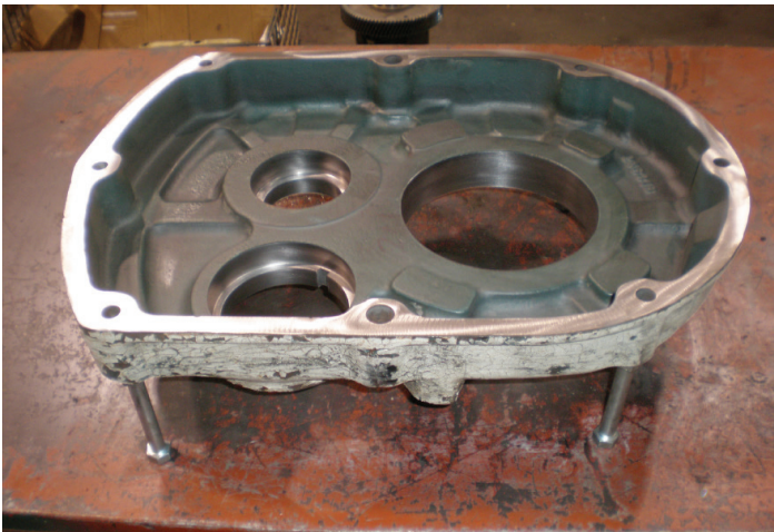
A returned unit must have a reusable housing (carcass) for it to be remanufactured as a future exchange unit
